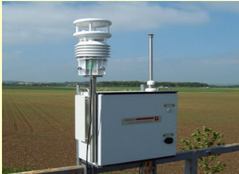
Optical particle counter measures PM_{2.5} and PM_{10} every 6 sec
